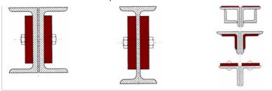
This fact sheet shows the example of the restoration and reinforcement of the Parc de la Tête d'Or greenhouses in Lyon. The original components dating from the 19th century were corroded and in places undersized; they had to be reinforced in accordance with the structure's architectural aesthetics and its status as a monument.
