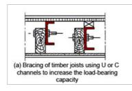
Figure a) shows an old floor reinforced with "trimmed joists". Steel beam reinforcement is performed using U-type channels, braced to limit the risks of warping and positioned on one or both sides of the piece to be strengthened. Defective joists, often warped, are secured to these new sections.
