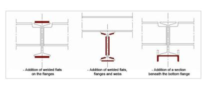
In the case of floors, reinforcement of the initial steel section is performed by the addition of steel flats and/or sections, which are fastened to the original beam by welding, bolting or bonding. This bracing is generally located beneath the bottom flange, or possibly on the web of existing sections. The top flange may also be reinforced when it is accessible.
