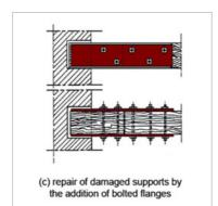
The problem is addressed by establishing a new support in the form of either corbels, columns or wall elements. A new piece of treated wood can also be joined to the defective joist by means of two steel flanges fixed by means of lag screws or by bolling.
